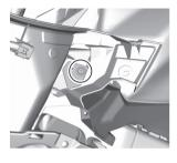
6. Remove the fasteners. The frame covers have fasteners behind the cover at the places marked with rectangles.
