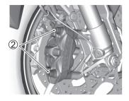
NOTE: Never squeeze the brake lever with the caliper removed. It is very difficult to force the pads back into the caliper assembly and brake fluid leakage may result.
